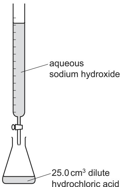
The end-point of the titration with each indicator occurs when  $23.6 \text{ cm}^3$  of aqueous sodium hydroxide is added.
